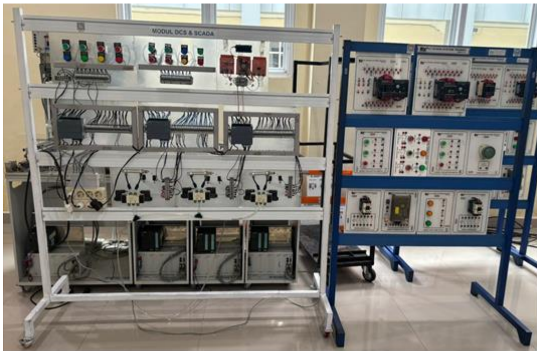
Gambar 3.4 sistem kontrol hardware terintegrasi (PLC, DCS &amp; SCADA, ESP32 IoT)
